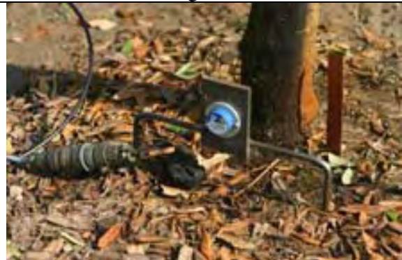
Inclinometer (with cable) measured angle of root ball as tree was pulled over.
