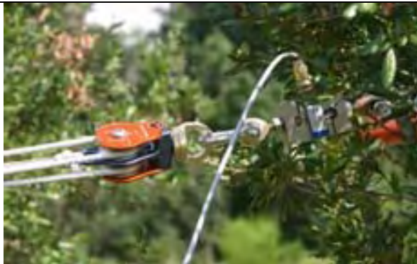
Pulley system with load cell and cable to computer to measure force.
